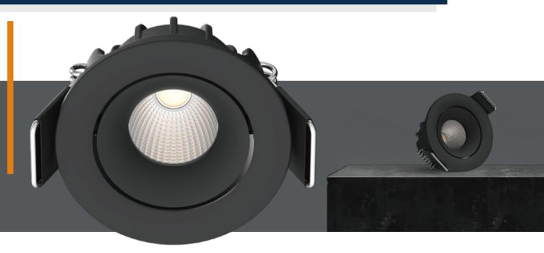
This Morro spot is available in fixed & tilt version, with a sturdy matt white and matt black finish. It has a diameter of only 50mm and is less than 35mm high. The Morro has a very compact driver that fits perfectly through the small recessed hole for the spot. Despite the dimension is small, the performance of this driver is great. The pressed aluminum housing not only has beautiful appearance, but also provides good heat dissipation.
