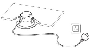
Hold back the spring clip and push the lamp in. Make sure the downlight is fixed tightly and properly in the ceiling.
