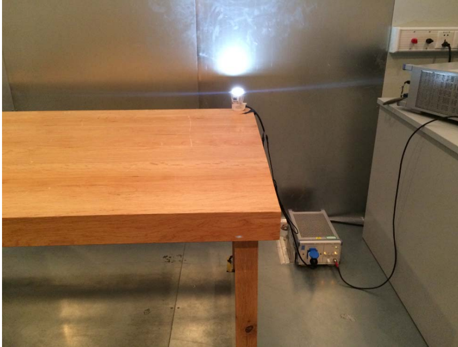
Mains Terminal Disturbance Voltage Measurement
