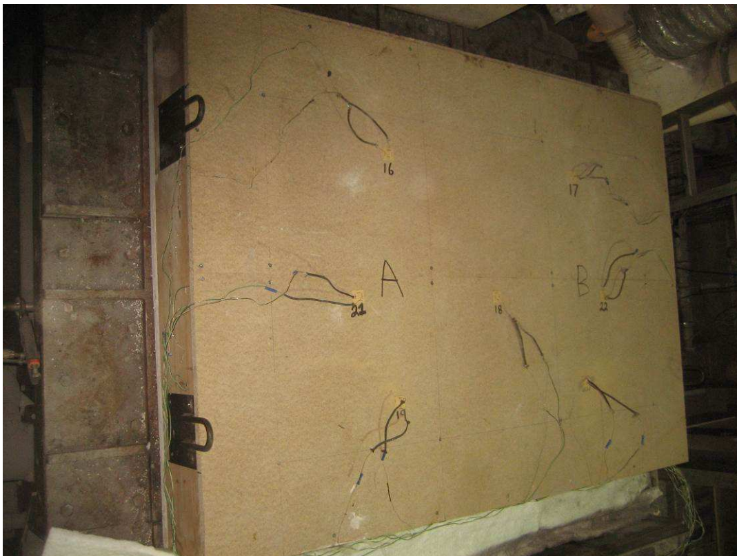
Photo 2.2.4 – Unexposed face after 80 minutes.
