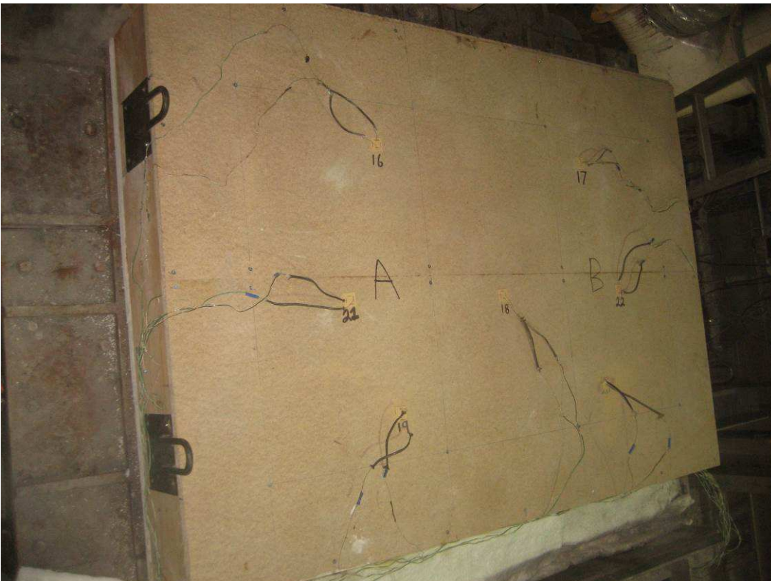
Photo 2.2.6 – Unxposed face after 99 minutes.
