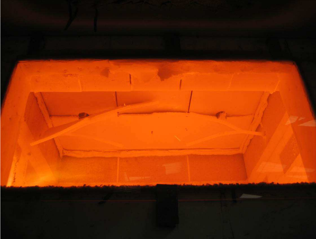
Photo 2.2.6 – Unxposed face after 99 minutes.
