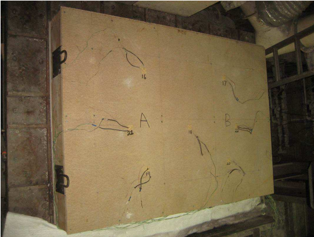
Photo 2.2.2 – Exposed face after 30 minutes.
